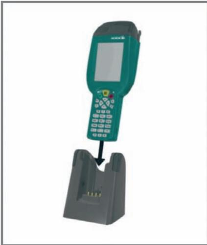
Fig.15 Placing the PL3000 to the charger
