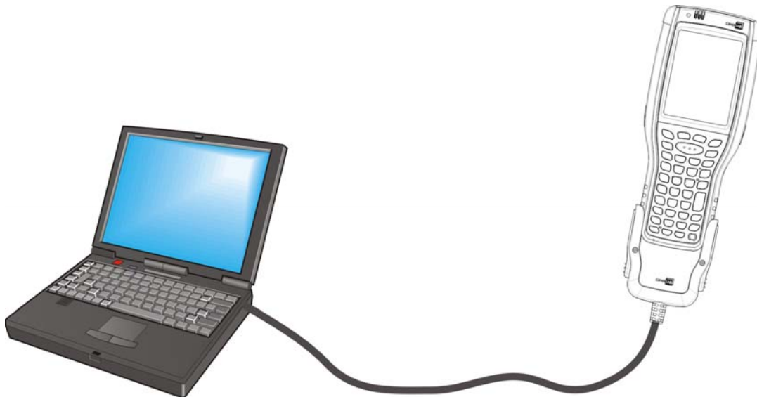
Figure 10: Direct Data Communication Using Snap-on Cable
